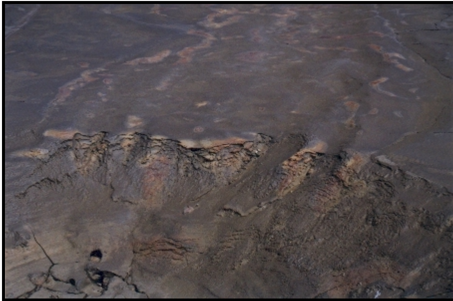
Oxidation of pyrrhotite in tailings soon after deposition.
