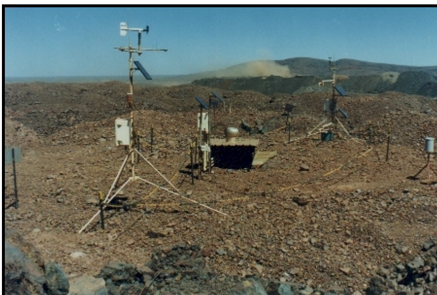
Equipment established at and below the surface of a waste dump at Mt Whaleback, WA, to monitor infiltration of rainwater into and evaporation out of the surface of the dump
