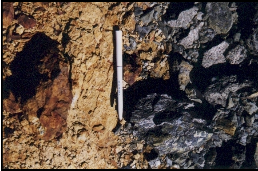
Pyrite on the left hand side has commenced reacting before pyrite on the right side. It is often difficult to estimate when pyrite oxidation will start to occur.
