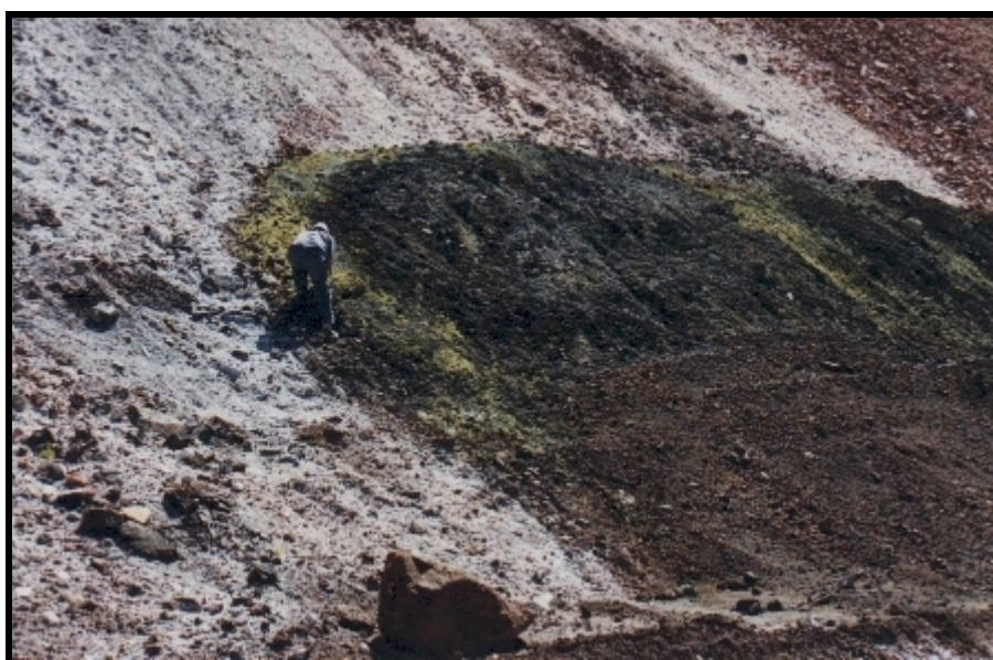
“Dry” oxidation (combustion) occurring at and near the surface of a waste rock dump.
