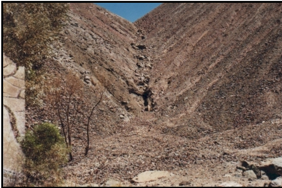
Coarse material depositing at the boundary of coalescing faces of an advancing waste dump – a preferred pathway forming for movement of oxygen and water.
