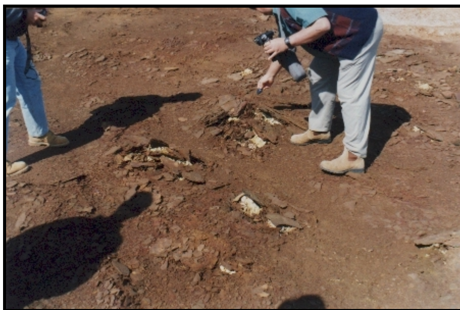
Venting at the surface of a pyrrhotite tailings deposit with precipitation of yellow sulfur.
