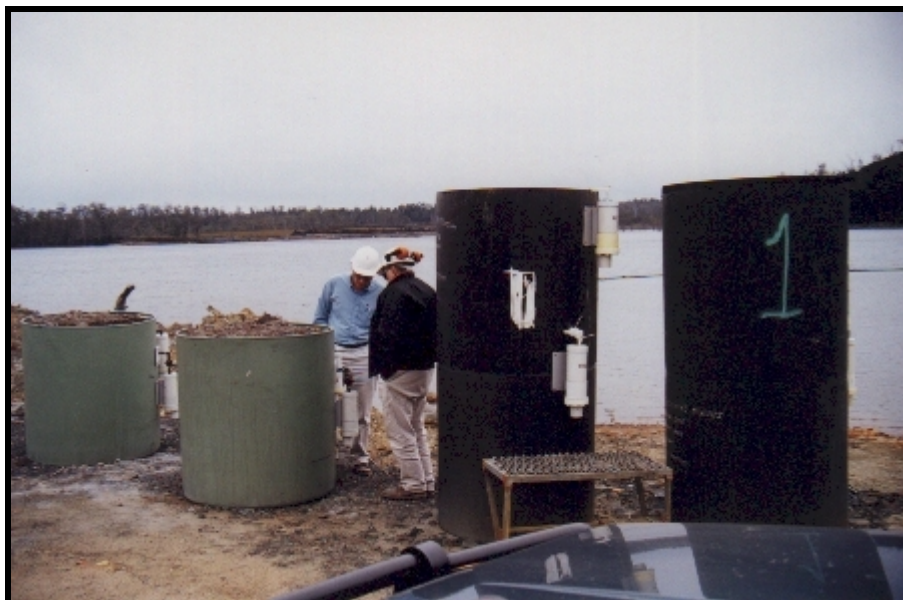
Kinetic testwork on tailings in plastic tanks.
